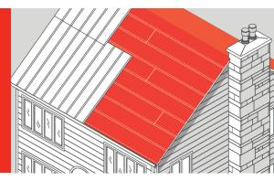
**High performance self-adhesive underlayment for metal roofs**, or as a perimeter membrane under one-ply roofing system and asphalt shingles. It is designed to withstand temperature variations from -45 °C to 126 °C (-49 °F to 260 °F).
