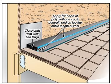
2. Apply 3/8" bead of polyurethane caulk (provided in box) beneath Roof-2-Wall Vent pieces and nail down with 2½" nails (provided), using a minimum three nails per piece. Run vent at least 6" past slot in decking and close off ends by inserting R2W End Plugs (provided) into end openings. Caulk End Plugs to roof and vent and seal ends after placement. Run another 3/8" bead of flexible caulk along the top of all vent pieces.
