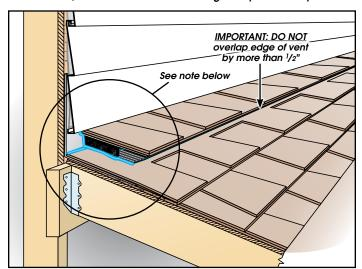
**4.** Cap or cover Roof-2-Wall assembly with shingle tabs or heavy gauge/decorative metal cap – cap should overhang the vent by a minimum of ½". Be sure to caulk all ends and joints to ensure a water-tight installation.\*
