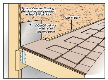
1. Start by cutting 1" a wide clear slot in roof deck at or near the top. Stop slot no less than 6" from the ends of the roof section to be ventilated.
