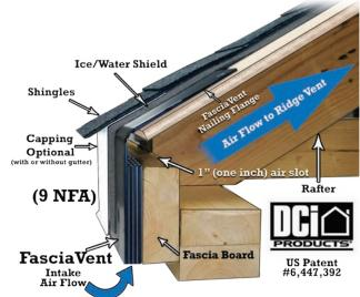
Note: a 1" air space between the roof sheathing and fascia boards & supports is required at the roof & fascia junction.
