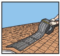
**3.** Beginning at end of ridge, apply vent with minimum 1¾" nails (2 coils provided in box) following "NAIL HERE" guides along vent cap. Only apply nails within the area between leg cavities – DO NOT apply nails outside of "NAIL HERE" guide marks. Vent may be power nailed or hand nailed. Do not overdrive nails. Apply first four nails (two on each side), then remove colored band to unroll rest of vent. Continue to apply according to marked guides.
