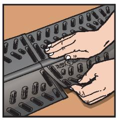
**4.** For runs longer than 20 feet, additional vent rolls can be applied. Line up end of additional vent roll with previous roll by overlapping at offset lip. **Follow Step 3** to apply rest of vent.
