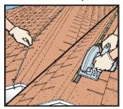
**1.** Measure a 3" slot,  $1\frac{1}{2}$ " each side of ridge centerline. This allows for a 2x ridge board or smaller. Snap chalk lines the entire length of the ridge. Cut slot with a circular saw and clean out debris. Set saw depth so as not to cut roof rafters. Stop the slot 12" short of any ridge end, intersecting ridge or obstruction (such as a chimney).
