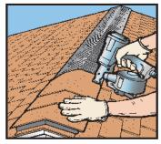
4. Continue to tack nail both sides of entire length of vent. Use nail pattern shown in step 3. Center shingle cap on vent and nail. Continue nailing until all vent is covered with ridge caps. Be careful not to overdrive nail. Nail head should be flush with top of shingle, without indenting it. Pre-forming caps in cold weather helps avoid cracking.
