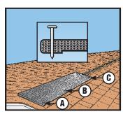
**3.** Fold flap under and secure with a 2" roofing nail. This allows the nail to penetrate an extra layer of vent material (inset). Align starter end ½" in from edge of roof, and centered on ridge. Be sure to caulk between bottom edge of vent and roof. Nail the starter section at points A, B & C, 2" up from edge.
