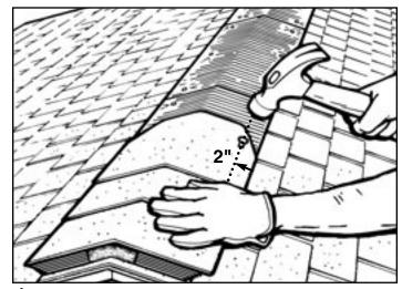
**4.** Center shingle cap on vent and nail. Nail line for cap shingles is to be  $2" - 2^{1/2}"$  up from edge. Continue nailing until all vent is covered with ridge caps. Be careful not to overdrive nail. Nail head should be flush with top of shingle, without indenting it. Pre-forming caps in cold weather helps avoid cracking.
