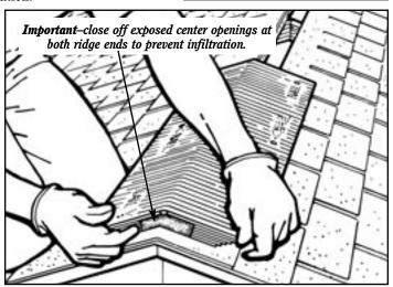
**2.** Nail one shingle cap at each end of the ridge, as with conventional application. Use End Plug in the exposed end on first and last sections of vent, caulk in place. Center first piece on ridge and nail, keeping end of vent ½" from end of roof. Set 4 nails ½" from ends and 2" up from edge on each corner of vent, add 2 nails in center of vent 2" up from edge. Repeat this step at the other end of the ridge. For V-300, use the Folded End Cap technique shown on back page.
