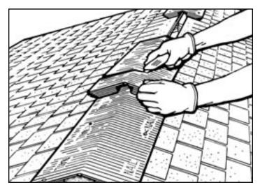
**3.** Continue applying COR-A-VENT, **working from ends to middle**. This technique helps remove any dips or sag in the ridge. Align center with previous pieces, making sure vent matches roof pitch before nailing. Continue nailing until entire ridge is covered. Use a utility knife to cut last piece to length. Caulk where bottom edge of end caps rest on roof.
