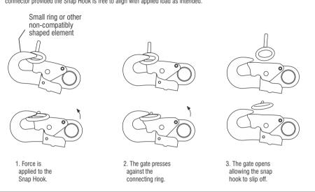
Making Connections: Only self-locking Snap Hooks and/or carabiners shall be used with this equipment. Ensure all connectors
