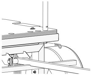
2. Secure the rolled goods rack by inserting the safety pin into the post hole underneath the cart frame.
