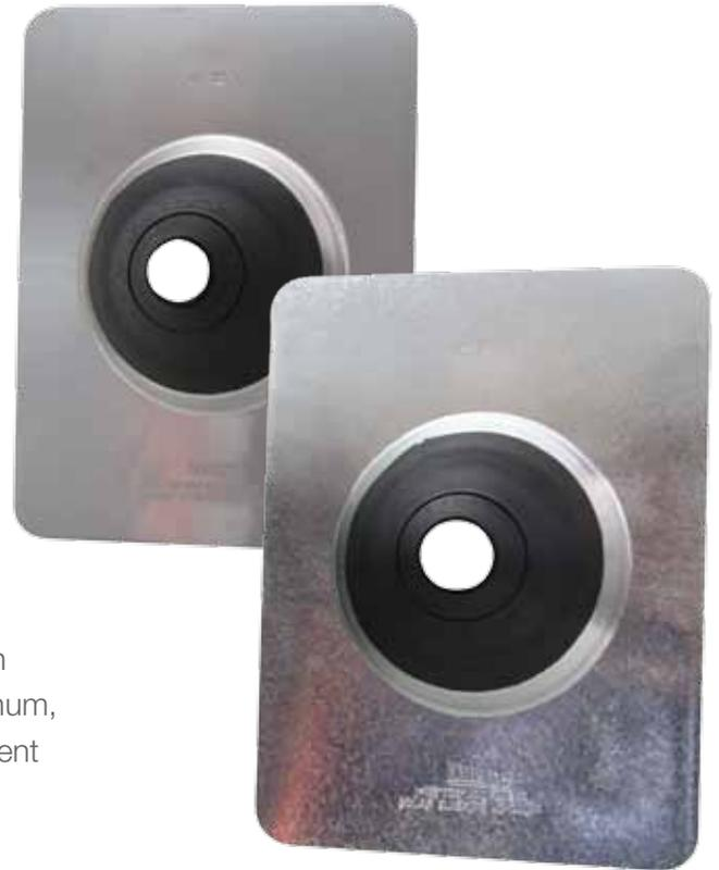
Oatey No-Calk® Solar Flashings are designed to flash around solar mounting systems. The products consist of a metal base with an elastomeric collar that incorporates a unique tear out feature enabling it to snugly fit most common mounting systems. The flashing bases are available in aluminum, soft aluminum or galvanized metal to accommodate all different roofing materials.
